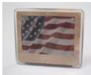
Figure 7. Active-matrix colour display
