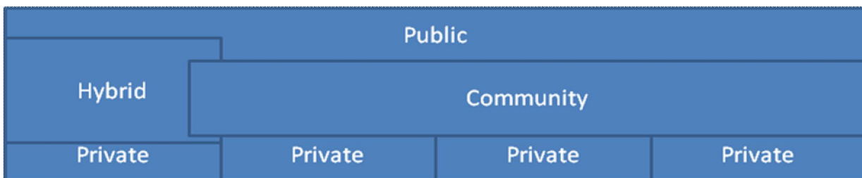
Figure A-1: The deployment models allow for a reasonable degree of interpretation. An organisation may have multiple Private Clouds, one of which can also be used by a Community; a Community Cloud may make use of multiple Private Clouds, and one which enables use of a Hybrid Cloud; Hybrid Clouds could variously combine Public, Private and Community at different times.
