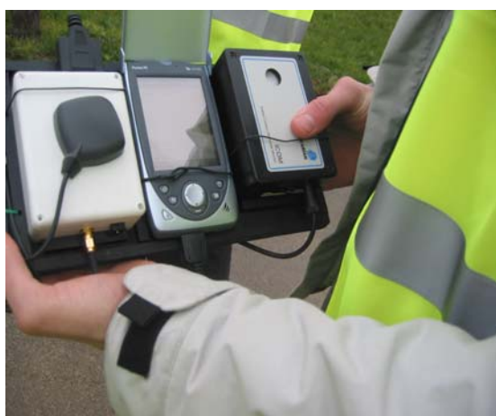
Fig. 4 CO monitor used in the Public Understanding for eScience project. With kind permission from Josh Underwood
