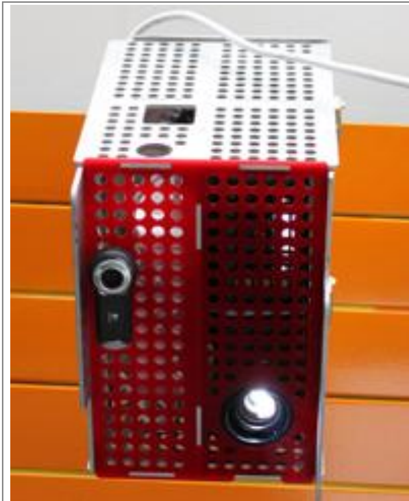
Pod containing Projector, Webcam, and Apple Mac Mini computer. Computer connects wirelessly to a server to support Podcast production and hosting. User can interact using Bluetooth mouse and keyboard.
